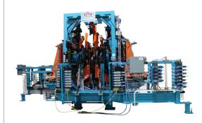
This large custom-built machine was designed to pierce and insert Spac® nuts in an automotive front cradle assembly.
