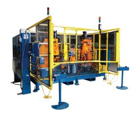
This custom dual workstation machine uses Tog-L-Loc $^{\scriptsize @}$  to assemble an automotive part.
